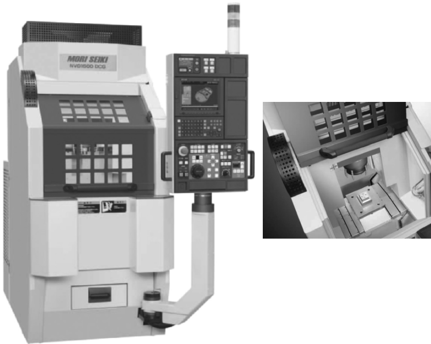
Figure 5.30. Mori Seiki milling machine, left, and with “box” open for access, right, courtesy of Mori Seiki.
