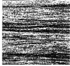
c. Hot rolled, 83% reduction, showing clear elongation and directionality
