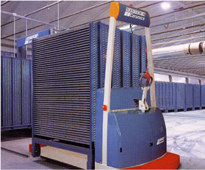
Fig. 4.10 An automated guided vehicle (AGV) transporting a box full of ceramic tiles
