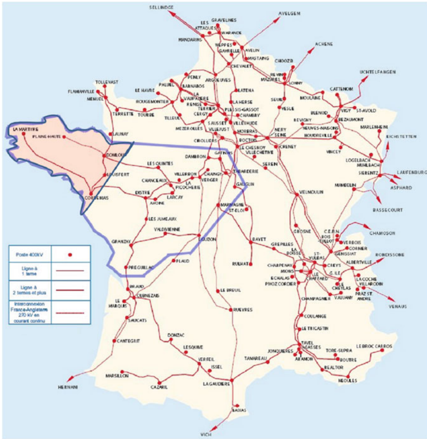
Fig. 10 French 400 kV network with SEO and Brittany highlighted
