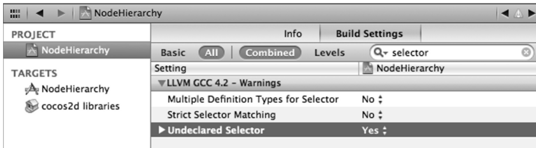
Figure 3-6. Activating the build setting to warn about undeclared selectors
