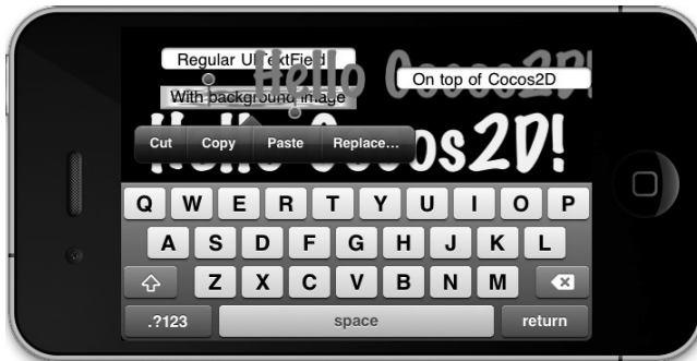
Figure 15–4. UIKit views on top and behind the cocos2d view, with input enabled for all of them
