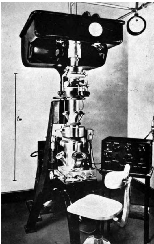
Figure 1-9. First commercial TEM from the Siemens Company, employing three magnetic lenses that were water-cooled and energized by batteries. The objective lens used a focal length down to 2.8 mm at 80 kV, giving an estimated resolution of 10 nm.
