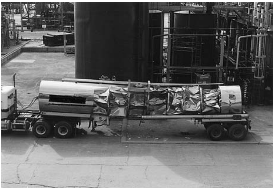
FIGURE 2-4 Side view of collapsed tank truck.
