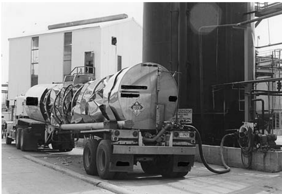
FIGURE 2-2 Collapsed tank truck with unloading hose connected.
