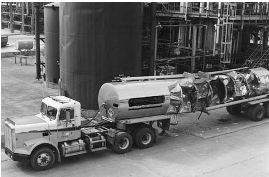
FIGURE 2-1 Tractor and collapsed tank truck at unloading station.
