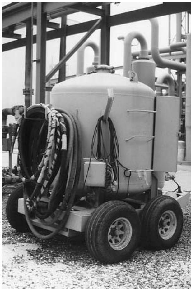
FIGURE 8-4 Repairs to a portable sandblast pot do not meet specifications and the lid flies off.
