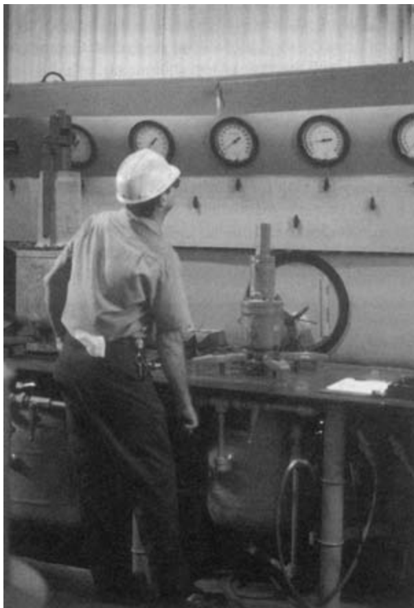
FIGURE 10-18 A well-trained mechanic testing a safety relief valve just as it is received from the unit.
