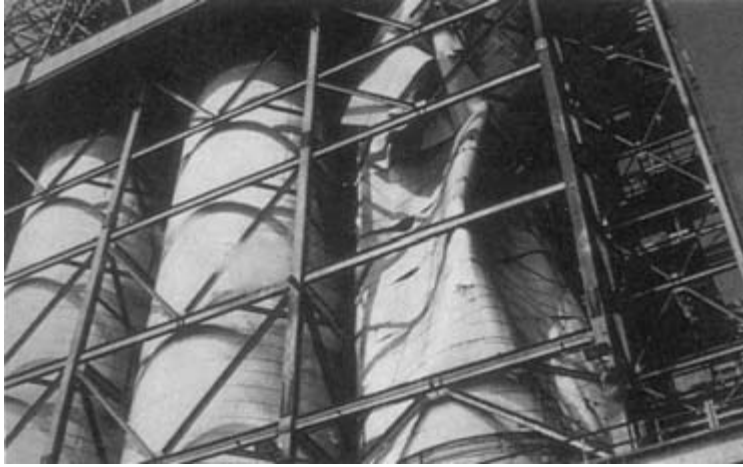
FIGURE 3–11 Close-up of the destroyed coker drum—crushed in like an aluminum beer can. Courtesy of S. O. Kapeniaks.
