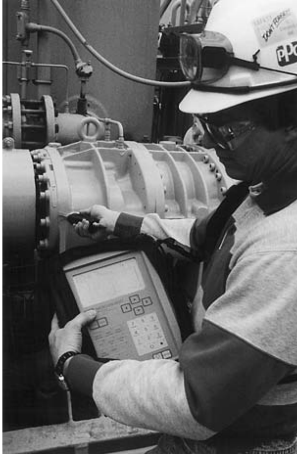
FIGURE 10-4 A close-up of a rotating machinery specialist with a vibration data acquisition module.
