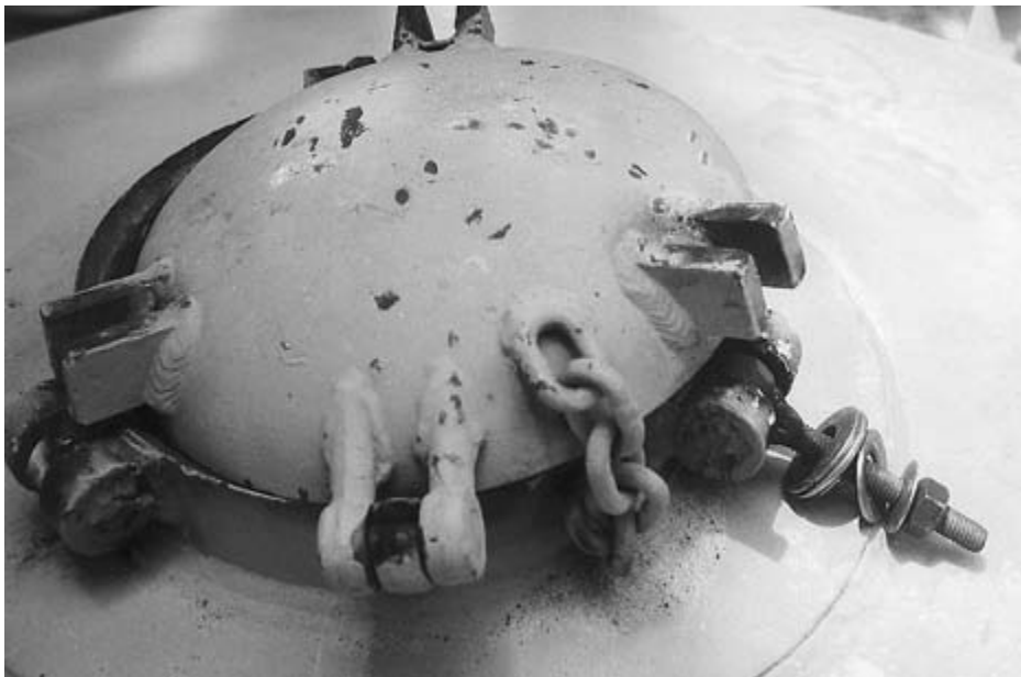
FIGURE 8-5 A close-up look at the quick closure bolts that failed on the sand pot.
