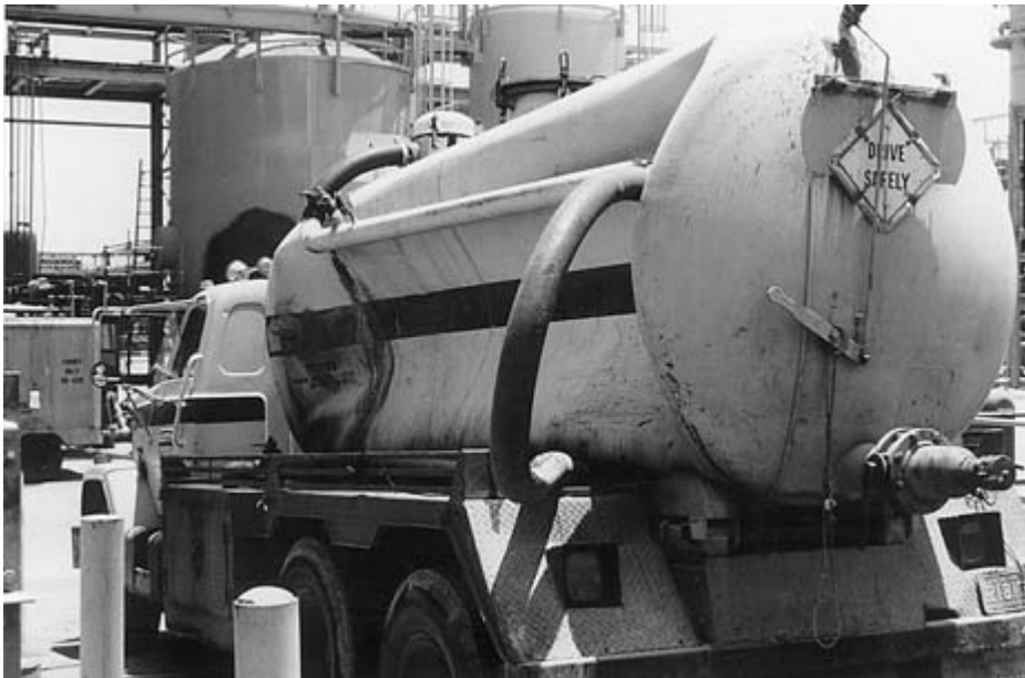
FIGURE 10–12 A collapsed service company vacuum truck signals an inadequate mechanical integrity program.
