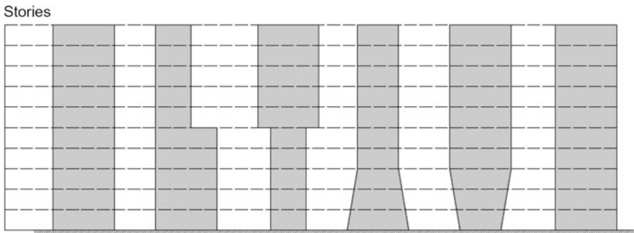
Fig. 21.43 Elevation configuration for shear walls
