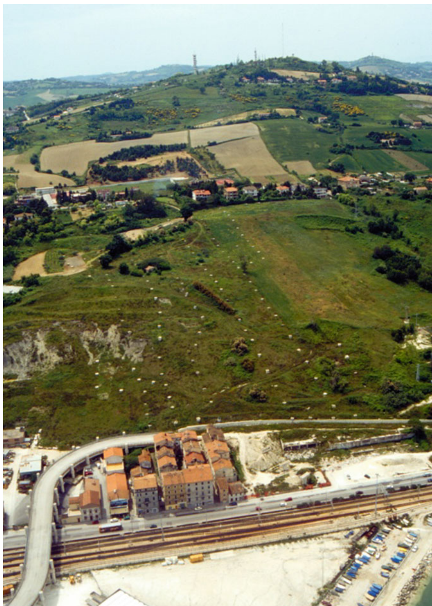
Fig. 7.9 Landslide area corresponding to the development of Section S–N. Four main trenches can be identified, with their scarps, parallel to themselves and to the coastline, which are typical of the front of every landslide
