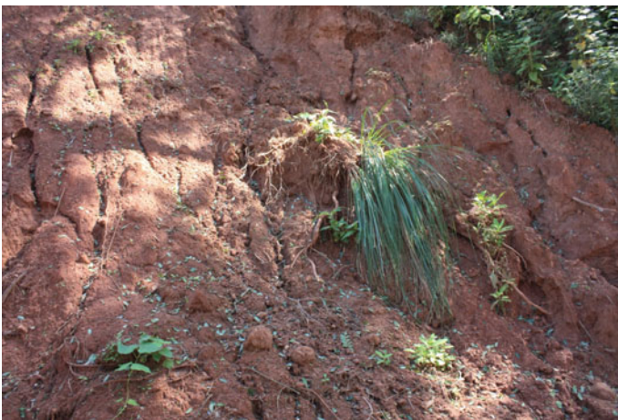
Fig. 5.27 Viscous-plastic deformation of the altered horizon
