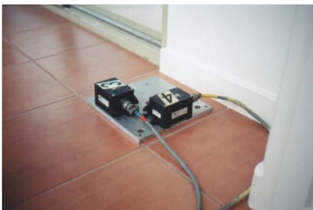
Figure B.5 Photo of accelerometer setup
