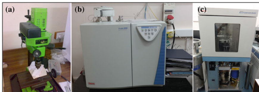
Fig. 3.13 a Triaxial drilling machine for isotopic analysis; b–c Isotope Ratio Mass Spectrometer (IRMS) coupled with a Kiel-IV automatic carbonate device at NGRI Hyderabad
