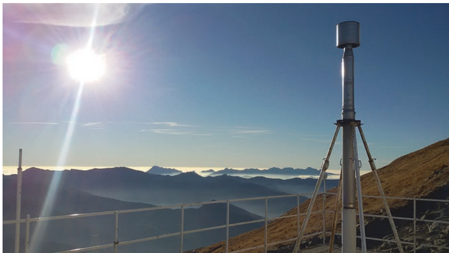
Fig. 7 External view of the sampling system for aerosol particles on the “O. Vittori” observatory terrace. The Apuan Alps can be seen in the background
