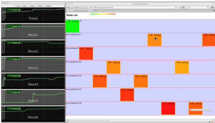
Fig. 3 Server Power (left) and VM Locations (right). The power consumption of the datacenter (shown in the upper left corner) was high, because heavily-loaded VMs were distributed to all physical servers.
