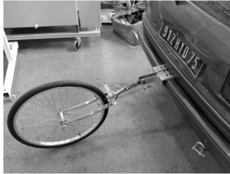
Fig. 2 Fifth wheel, or drive wheel.
