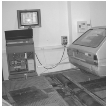
Fig. 1 Test 1 measuring on the brake roller tester at the MOT centre.
