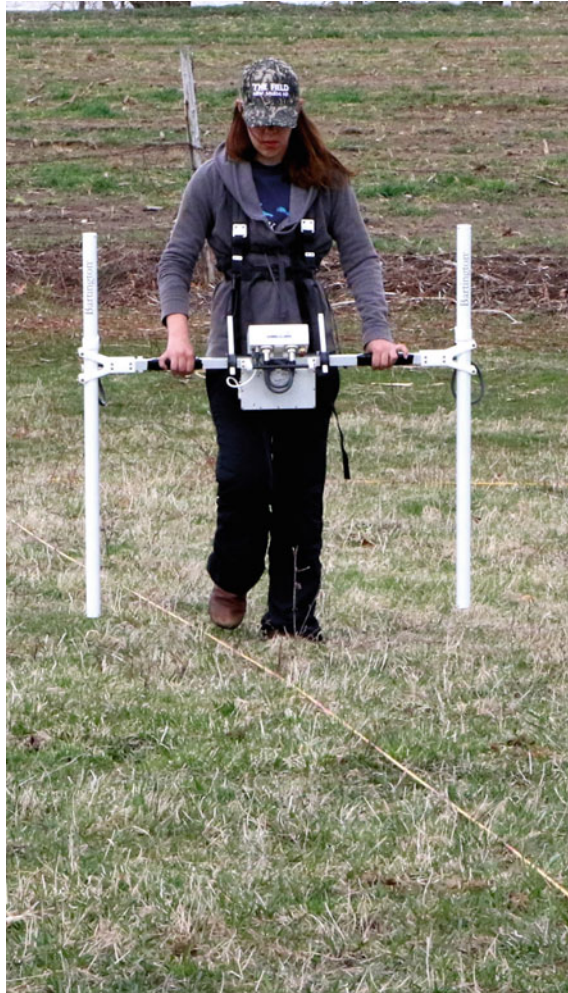
Fig. 3.2 A Bartington dual sensor magnetic gradiometer system
