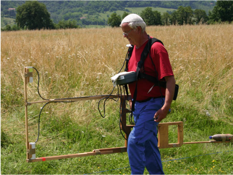
Fig. 3.7 Cesium gradiometer with two sensors, supported by a homemade carrying device constructed by Helmut Becker for ease of packing and traveling
