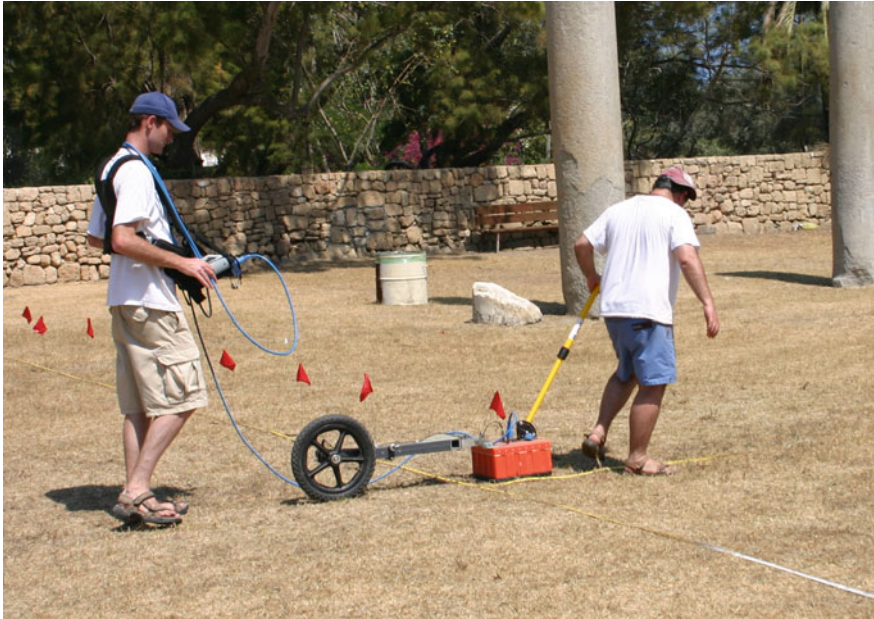
Fig. 2.2 A GSSI SIR-3000 GPR system with a 400 MHz antenna and survey wheel
