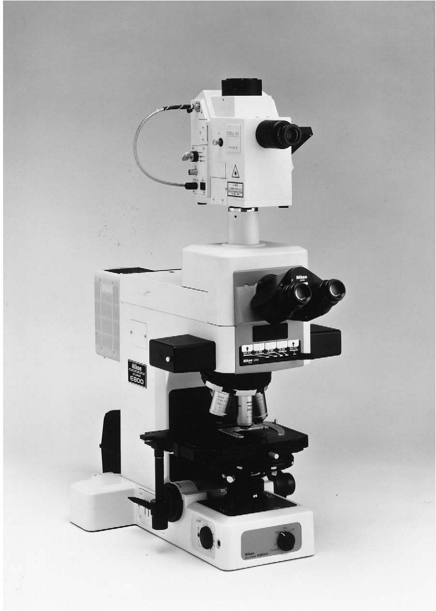
Fig. 1 The CSU-10 confocal scanning unit attached to the C-mount video port on top of an upright microscope (Nikon E-800). The scanner can also be attached to the video port of an inverted microscope. Illumination is conducted through a polarization-maintaining optical fiber from the laser source (not shown). (Figure courtesy of Yokogawa Electric Corporation.)
