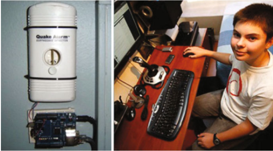
Fig. 7.13 A 14-year-old Chilean teen who created an earthquake warning system based on Arduino
