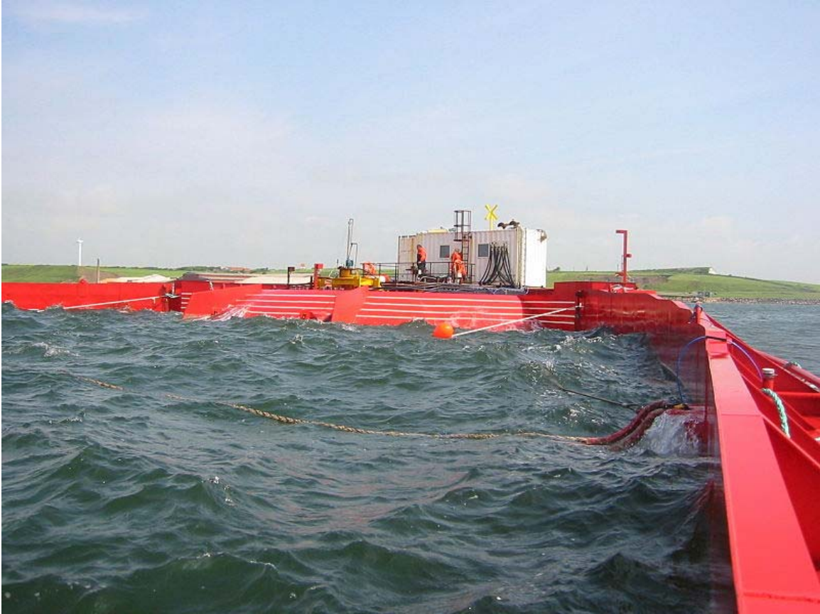
Wave Dragon seen from reflector, prototype 1:4½
