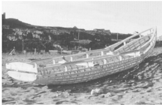
1 The skeletal structure of the curragh on inisheer, Aran Isles. (Photograph Peter Salter)
