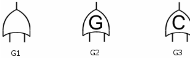
Fig. 5 Gates: G1 - the logical OR gate of digital circuits, G2 - the generalization OR gate of the profile, G3 - the causal OR gate of the profile
