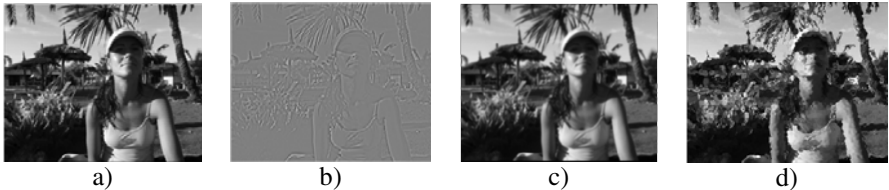
Fig. 2.1 The reference image (a) after: High Pass filtering (b), Gaussian Blur filtering (c), Glass filtering (d).
