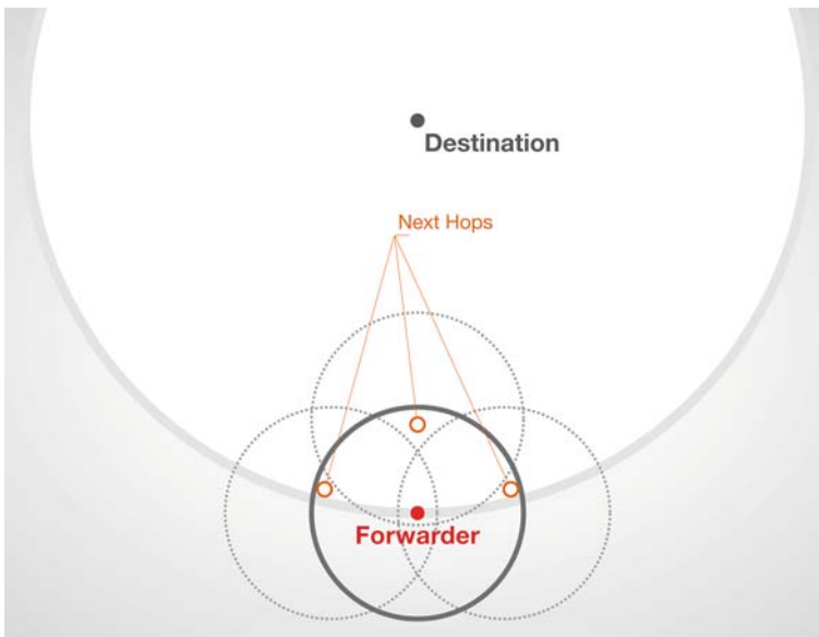
Fig. 5.6 Forward the same message from multiple nodes [7]
