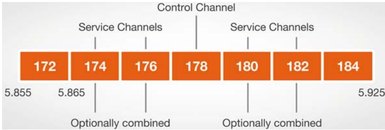
Fig. 7.1 DSRC frequency band allocation in US [3, 12, 13]
