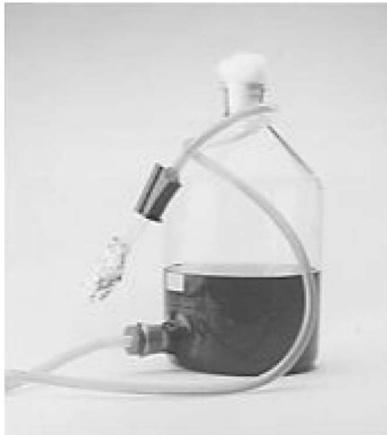
Fig. 1.7 Aspirator bottle with cell suspension, mounted with sterile tubing, tube connector and clamp.
