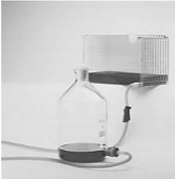
Fig. 1.16 To empty the Cell Factory, place it above the aspirator bottle, in the position shown, and the liquid will run out. Alternatively, the liquid can be poured out of that port into a waste beaker.
