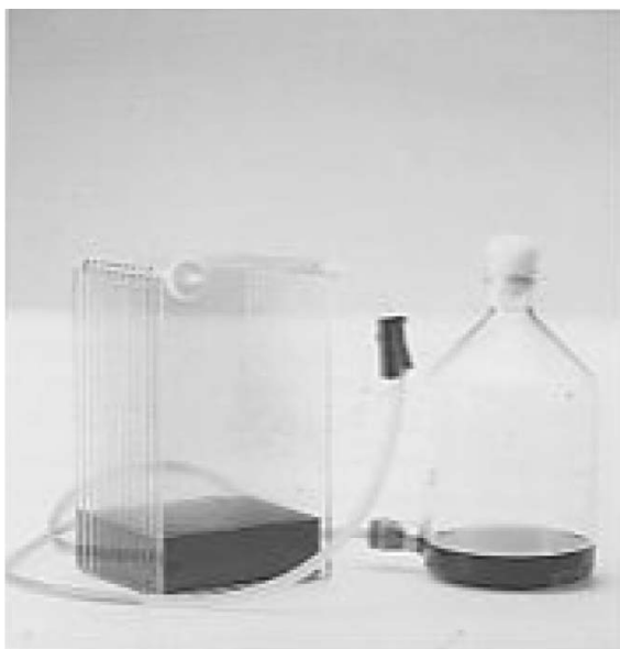
Fig. 1.13 Turn the Cell Factory 90°, putting the filling inlet up. The medium will be separated, with equal amounts of medium in each chamber.
