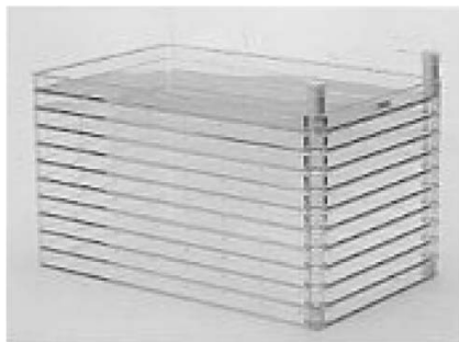
Fig. 1.3 Unpack the Cell Factory and place in a laminar air flow cabinet to work under sterile conditions.
