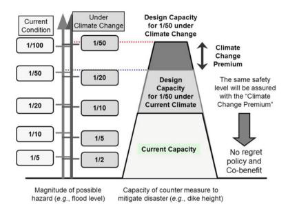
Fig. 2 Illustration of the impacts of climate change on the design level in water resources management. Safety level will be reduced when the same magnitude of hydro-meteorological hazard will occur more frequently due to changing climate, and the same level of safety will be assured by some increased adaptation capacity, referred to as "climate change premium". In the regions vulnerable for current climate variability, increasing the safety level has low potential to cause regrets in the future
