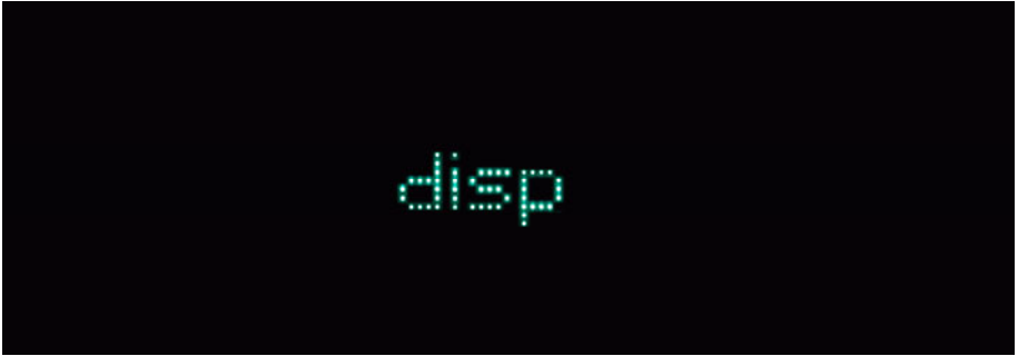
Fig. 2. The emission image of fabricated small-type triode FED panel
