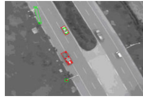
Fig. 9. At third clustering: The singular points are clustering for two clusters: vehicle and the noise.
