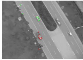
Fig. 8. At second clustering: The singular points are clustering for two vehicles with few noise.
