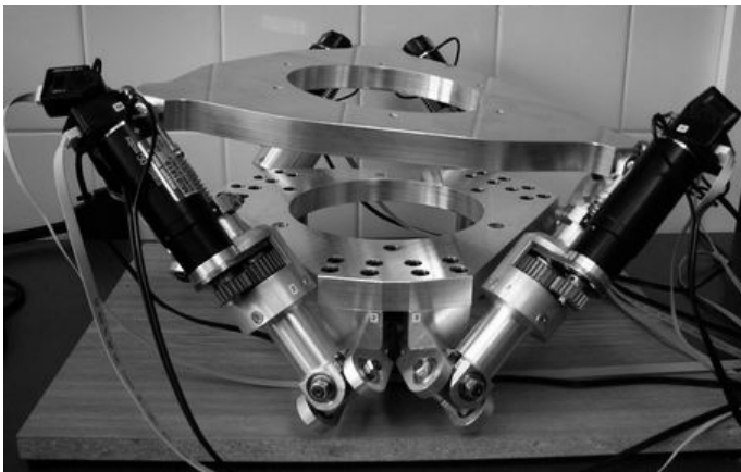
Fig. 2. The Stewart platform prototype
