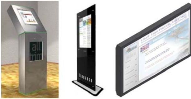
Fig. 1. Forms of the touch panel: free standing, desk and wall mounted.
