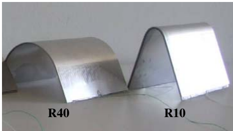
Fig. 2. Piezo-metal-compounds bended with different radii (40 mm and 10 mm)
