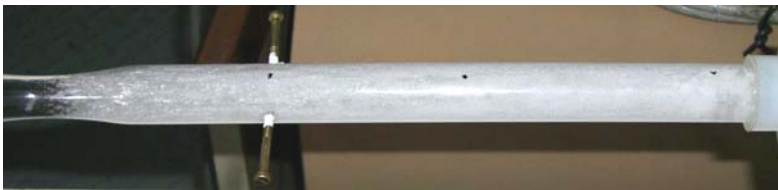
Fig. 7. The cavitation cloud (Pochylý, Fialová, Kantor [4])
