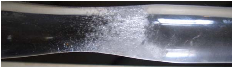
Fig. 6. The cavitation bubbles creation (Pochylý, Fialová, Kantor [4])
