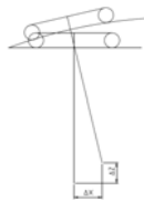
Fig. 5. Visualization of the error TCP in axes X-Z.
