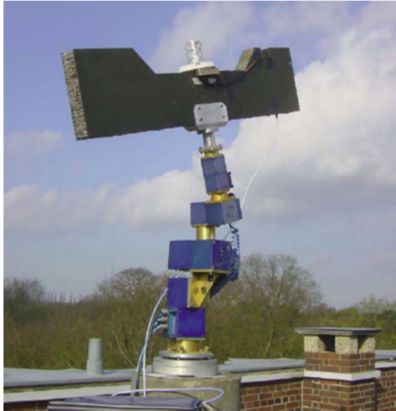
Fig. 13.1 GOCE GPS antenna set-up for near-field multipath calibration using a GOCE mock-up as originally proposed to ESA (GOCE Project Office) in (Švehla and Rothacher 2004b). (credit ESA)
