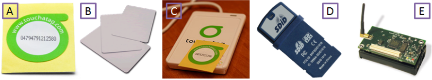
Fig. 2 Binary proximity sensors used in our lab deployment: A), B) passive RFID tags, C) RFID reader with USB interface, D) embedded RFID reader and E) MicaZ mote.
