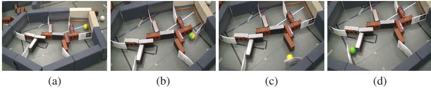
Fig. 23.4 A basic navigation experiment: a) the weasel ball is placed initially in the upper right corner; b) after 25 seconds it changes regions; c) after 32 it changes again; d) after 45 seconds it reaches its destination
