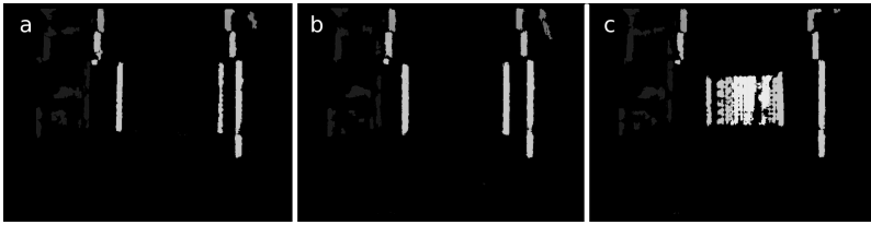
Fig. 11.5 Disparity images obtained using STOC camera (Videre Design) from 1000 mm: (a) white cardboard, (b) black cardboard, (c) chessboard. For the distance of 155 mm there is no information on the pictures while the whole field of view of the camera is covered by the uniform colour cardboard. There are no features for obtaining the disparity map.
