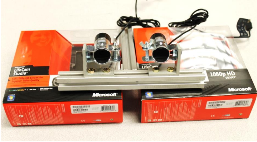
Fig. 6. LTU stereo vision camera developed with two webcams and Emgu CV
