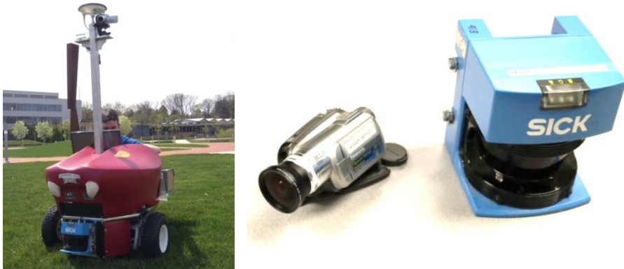
Fig. 4. Viper robot vehicle with a camera and a SICK laser rangefinder
