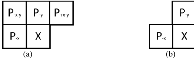
Fig. 7. Left: 4 point detection grid and Right: 2 point detection grid for connected component labelling
