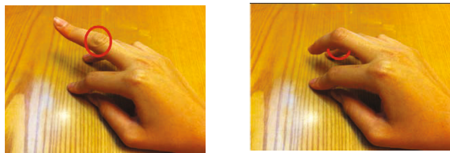
Fig. 4. Right click: like standard mouses right click, sensing whether right flexible sensor is bent or not is in charge of right click
