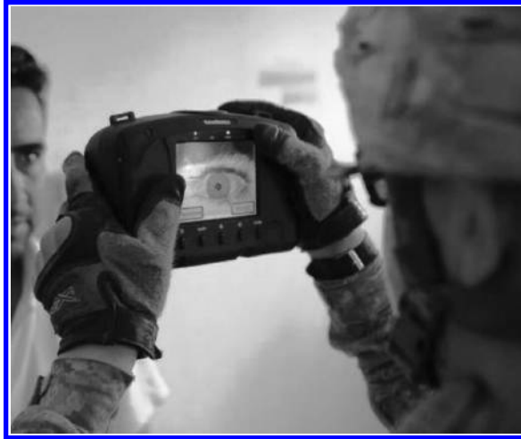
FIGURE 8.7 Handheld Interagency Identity Detection System (HIIDE). (Courtesy of the US ARMY [Sgt. Barrell, US ARMY, 2009].)
