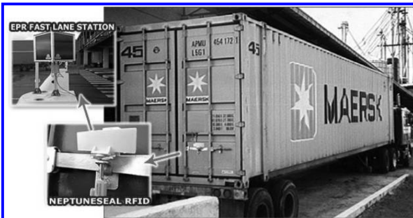
FIGURE 8.8 RFID technologies for container seals. (Courtesy of Maersk Lines.)
