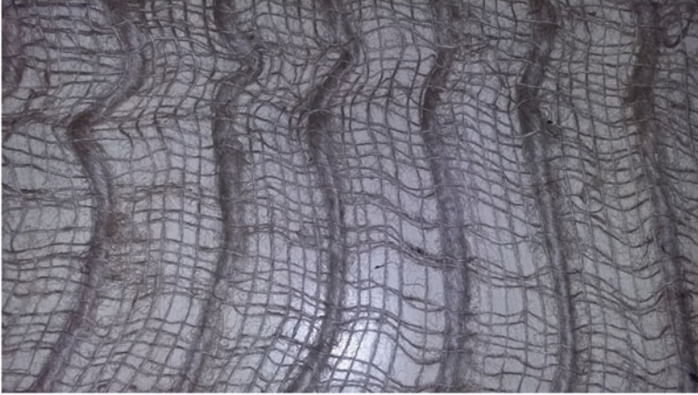
Fig. 15.2 Specially designed open weave JGT for wind erosion control in deserts
