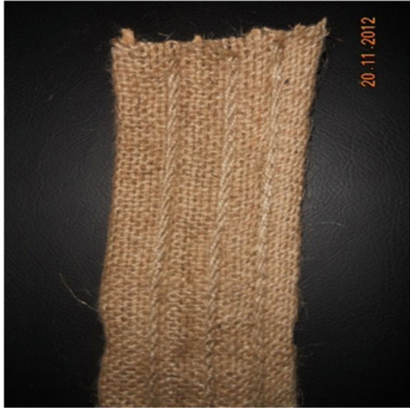
Fig. 10.1 Typical PVJD with coir wicks
