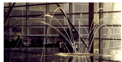
Figure 10.4: The water runs in continuous streams. Some fancy valve work (under the visible part of the fountain) is required to get such a laminar stream that holds together for the whole flight. This water draws its own graph of the trajectory of its particles. You can do the same kind of thing with a squirt gun next to a blackboard.
