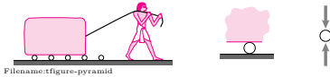
Figure 4.20: Dragging a heavy stone on rolling round logs. If there is only point contact between the logs and the ground and stone, the logs are two-force bodies. If the logs are also round there is no resistance to forward motion.
