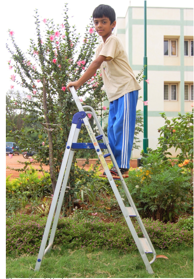
Figure 5.43: A ladder is well modeled as a collection of rigid pieces connected by pin joints ...
