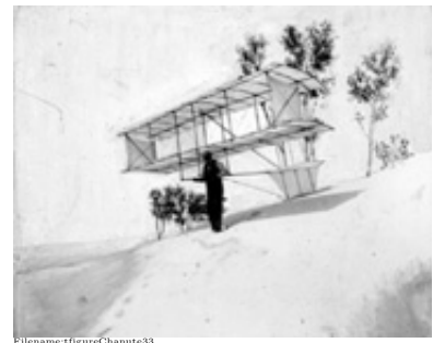
Figure 5.3: Chanute Glider, 1897. The Wright brothers first planes were near copies of the planes built a few years earlier by Octave Chanute, a retired bridge designer. Structurally these early biplanes were essentially flying bridges. The Wright brothers were preoccupied with trusses. Their first inspiration and main airplane patent was about how to control the distortion of a truss ('wing warping'). The Wrights even thought of the threads in their wing fabric as bars in a truss. Take away the outer skin from many small modern planes and you will also find trusses. (National Air and Space Museum Negative IA-2036084-10697)
