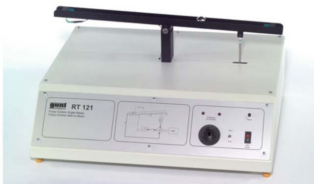
Fig. 4 1-dimensional seesaw model
