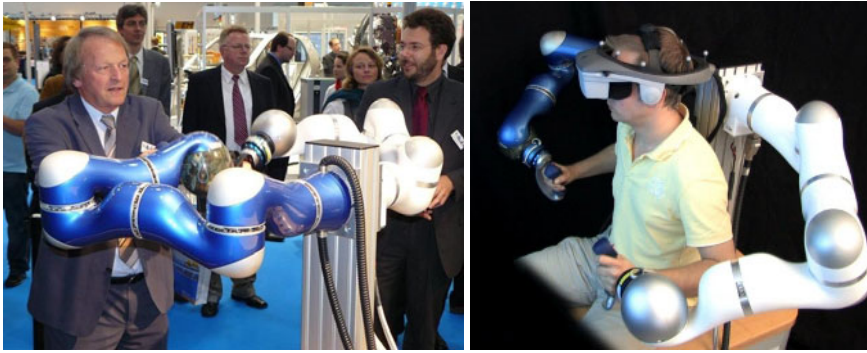
Fig. 5.6 A system with two robot arms attached to a common base provides bimanual haptic feedback. Two fundamentally different setups can be distinguished (left) the standard configuration, and (right) the ergonomic configuration of the bi-manual haptic interface.
