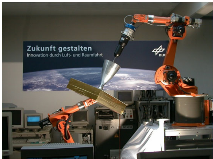
Fig. 6.10 The ESS demonstrator simulates the approach and docking of a robot arm to a tumbling satellite. A Kuka industrial robot approaches a satellite and captures it using the capture tool developed at the DLR.
