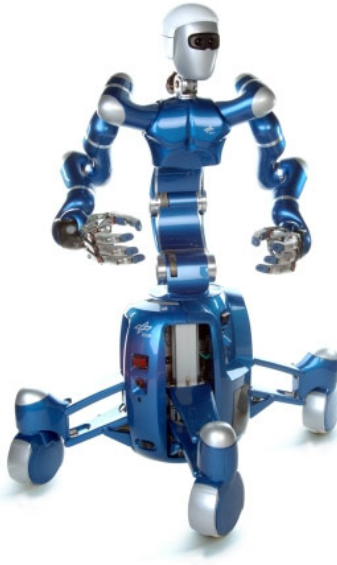
Fig. 6.2 The DLR mobile humanoid robot Rollin' Justin . Two DLR LWR arms are attached to an upper body. The omni-directional mobile base has a variable foot print.
