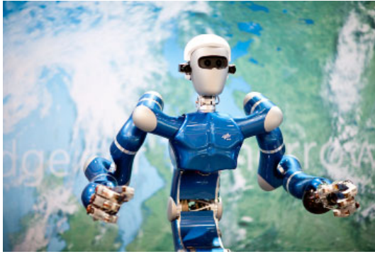
Fig. 6.15 DLR humanoid robot Justin looks quite human-like and friendly when the arms are in a configuration that appears comfortable for a human. Justin can move in a very human-like manner, but it can also perform movements that look very awkward for a human observer.
