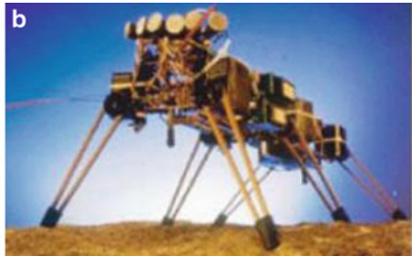
Fig. 1.9 DANTE-II, an eight-legged robot for volcano exploration [33]
