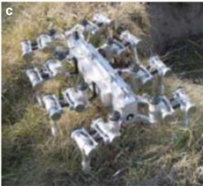
Fig. 1.10 Biologically inspired multi-legged robots. (a) SCOUT-II [37], (b) Genghis [33], (c) SCORPION [33], (d) AIBO [22]
