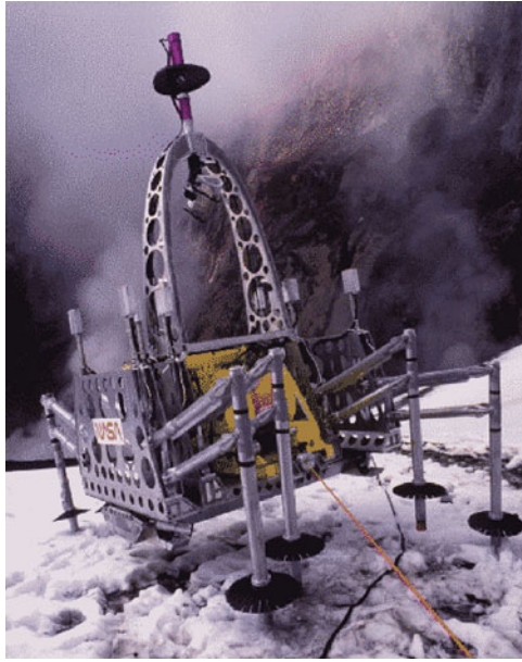
Fig. 1.9 DANTE-II, an eight-legged robot for volcano exploration [33]
