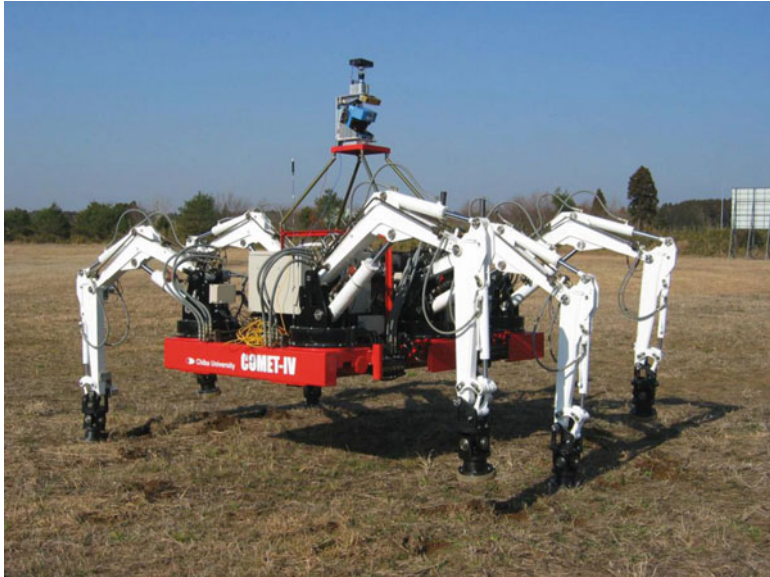
Fully autonomous walking robot COMET-IV: Walking mode
