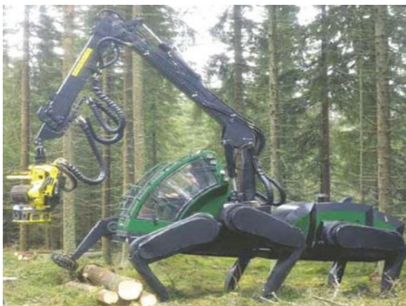
Fig. 1.8 Plustech, the forest-cutting machine employing legged locomotion [10]
