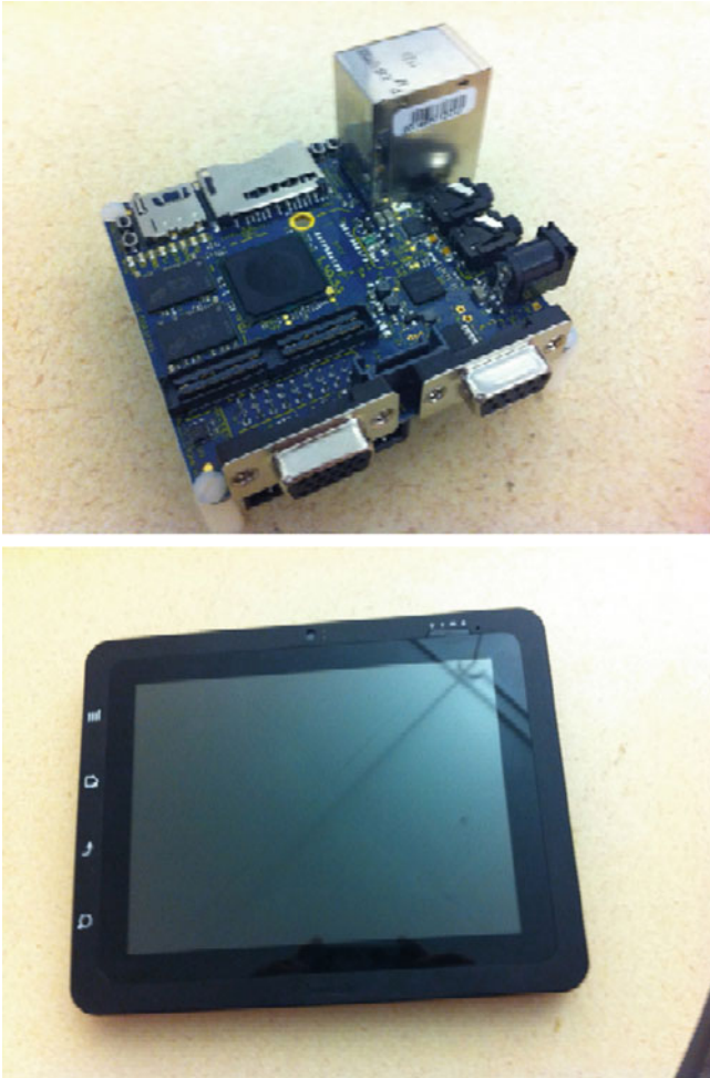
Fig. 4.6 FreeScale i.MX53 Development Kit: includes a development board and a tablet form-factor, both running the Cortex™-A8 ARM processor with TrustZone™ (split-world) isolation enabled
