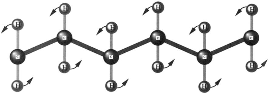
FIGURE 1.7. Mobility of hydrocarbon chain. The diagram shows mobility of a polymer chain composed of carbon atoms attached by single bonds with hydrogen side chains. Rotational freedom of the single carbon-to-carbon bonds allows hydrogen atoms to rotate freely about the backbone.
