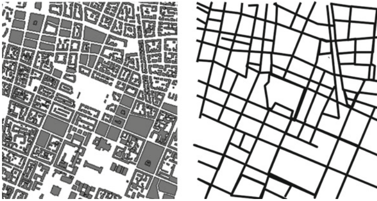
Fig. 3.18 Representation of a dense urban environment ( left , building geometry from Mannesmann Mobilfunk GmbH (1999)) as a graph with edges weighted by length ( right )
