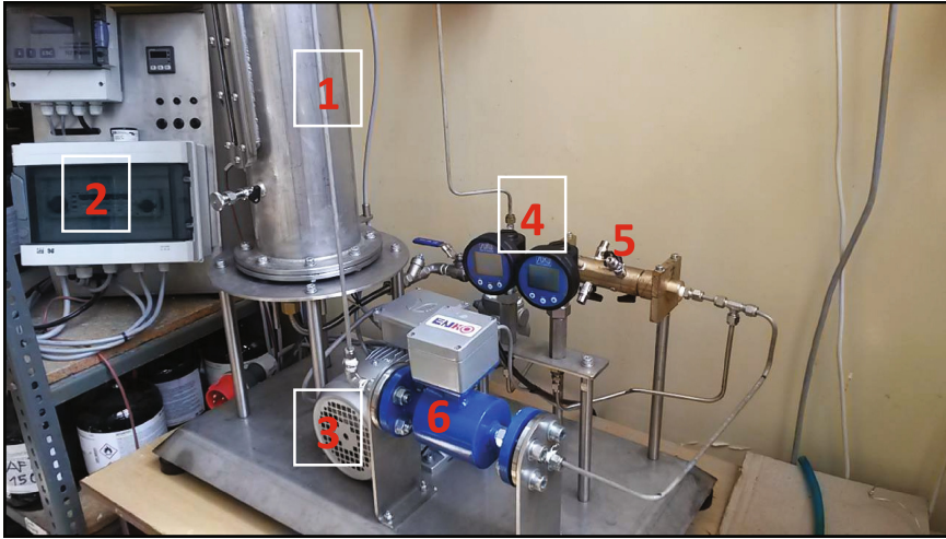
Fig. 2. A hydrodynamic cavitation reactor. 1 - effluent tank, 2 - control panel (mixing, temperature, volumetric flow), 3 - pump for effluents, 4 - pressure control, 5 - Venturi tube, 6 - flow control
