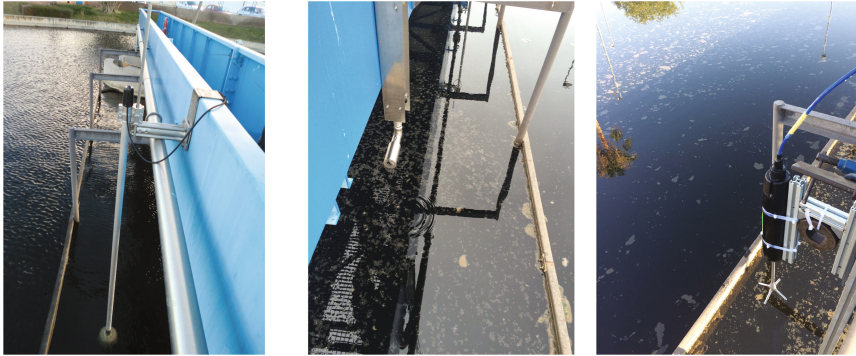
Fig. 1. Sonatex®, Solitax® and Vectrino® probes installed in a full-scale SST
