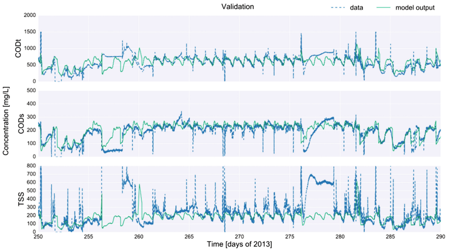
Fig. 2. Validation results for the influent model used to predict influent concentrations. From top to bottom: Total COD, Soluble COD and Total Suspended Solids concentrations. Validation happened on data from September 7 th to October 17 th , 2013
