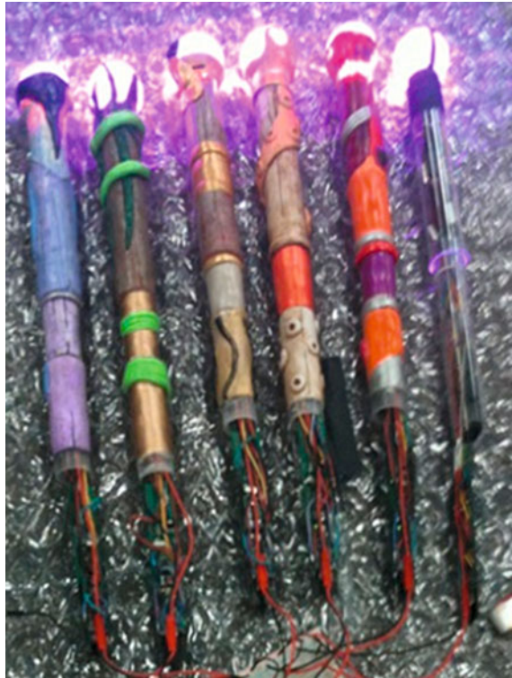
Fig. 16 Wireless gyro- and accelerometer-enabled wands for theatrical performance. (Courtesy of beaudry interactive)
