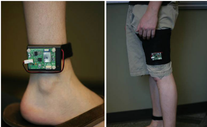
Fig. 6 Accelerometer placement for the real-time simple activity recognition system
