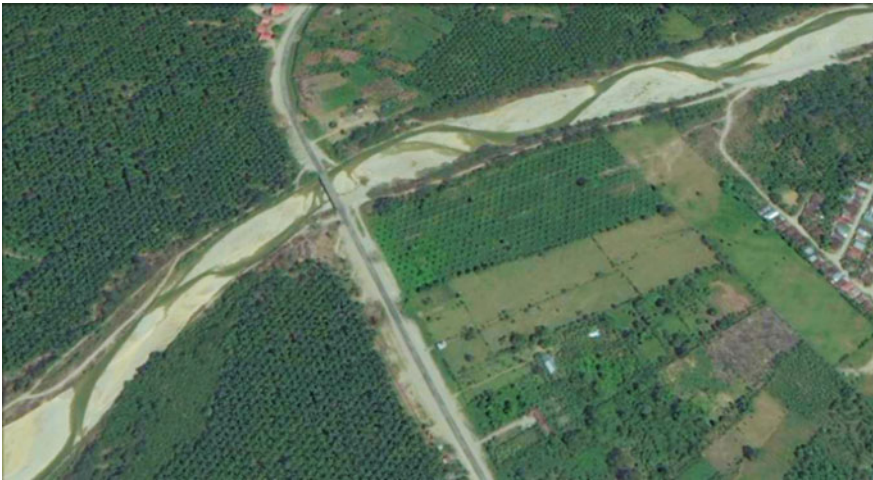
Fig. 1 Alternate bars in the Rio Coto, Costa Rica; flow from left to right (from Google Earth; photo source: Digital Globe; imagery date: 3/4/2015)
