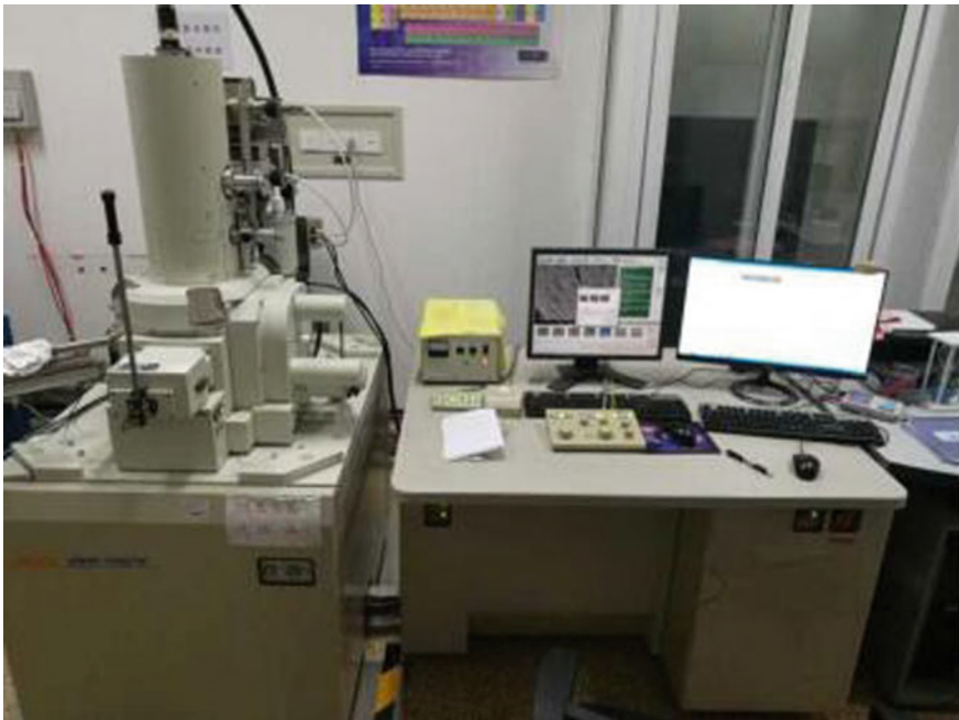
Fig. 2.8 Field emission scanning electron microscope and energy spectrum analyzer
