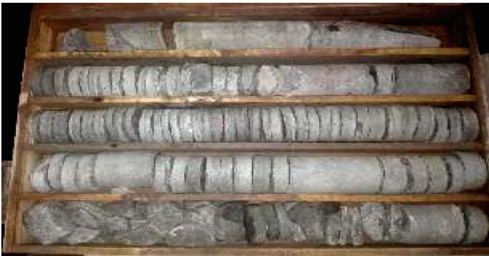
Fig. 8. Core samples showing disking
