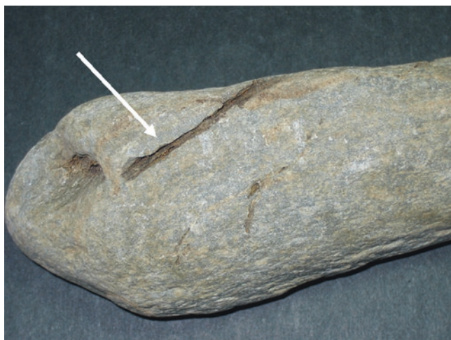
Fig. 7.2 Cavity formed through preferential mineral dissolution in a rock matrix
