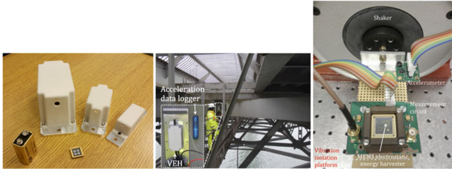
Fig. 6.17 Application example of environmental power generation by vibration using the concept of parametric excitation
