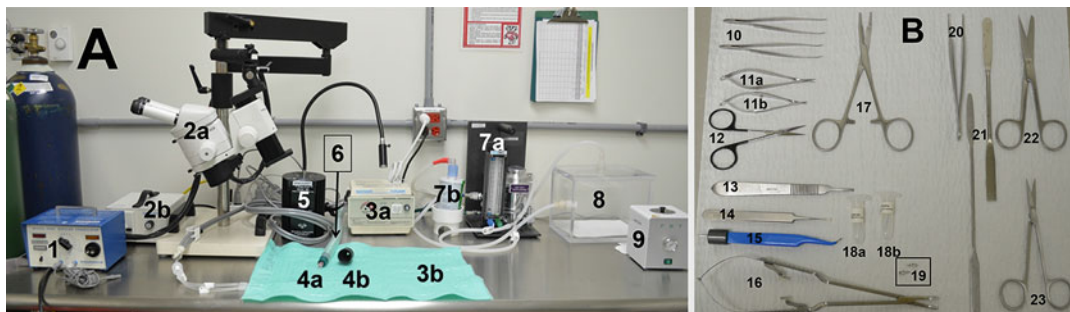
Fig. 1 Surgical area and equipment for MCAO. (a) Surgical table with anesthesia rig. Equipment pictured: (1) Electric cauterizer (Radionics, Model 440E bipolar coagulator). (2a) Surgical microscope (Leica MZ6). (2b) Light box for surgical microscope. (3a) Warm water blanket (Stryker TP22C). (3b) T-pump system (Gaymar T/Pump T-500). (4a) Mouse nose cone (Vetequip). (4b) Rat nose cone (Vetequip). (5) Prehensile light source (Dolan Jenner, Fiber-lite 190). (6) Bain circuit (Surgivet). (7a) Isoflurane vaporizer (Surgivet). (7b) Isoflurane charcoal filter (Vetequip). (8) Induction chamber (Surgivet). (9) Bead sterilizer (Fine Science Tools, #18000-45). Additional equipment is described in Subheading 2.1. (b) Surgical tools for MCAO and transcardiac perfusion. Tools pictured: (10) Pair of curved, extra fine Graefe forceps (Fine Science Tools, #11152-10). (11a) Vannas large microscissors for sharp dissection (Fine Science Tools, #91500-09). (11b) Vannas small microscissors for arteriotomy (Fine Science tools, #15000-00). (12) Iris scissors (Fine Science Tools, #14058-09). (13) Scalpel holder (blades not pictured) (Fine Science Tools, #10003-12). (14) Straight, extra fine, sharp-tip forceps (Fine Science Tools, #11295-10). (15) Cauterizing forceps (Radionics). (16) Microsurgical clip applicator (Mizuho, #07-942-02). (17) Needle driver (Fine Science Tools, #12002-14). (18a) MCAO filaments for mice (Docol, #6023). (18b) MCAO filaments for rats (Docol, #403934). (19) Microsurgical clips (Mizuho, #07-940-56). (20) Rat-toothed forceps (Fine Science Tools, #91127-12). (21) Spatulae. (22) Sharp/blunt surgical scissors for rat perfusion (Fine Science Tools, #14001-13). (23) Fine, pointed surgical scissors for mouse perfusion (Fine Science Tools, #14068-12). Additional detail on certain tools can be found in Subheadings 2.3 and 2.5. Some tools not pictured are described in Subheadings 2.3 and 2.5
