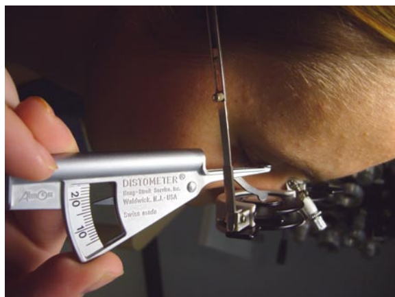
Fig. 2.4 A Distometer (Haag-Streit Services, Waldwick, N.J.) is used to measure the vertex distance in a patient with high hyperopia while wearing trial frames
