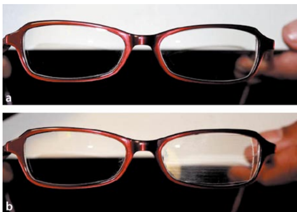
Fig. 16.8a,b Straight-edge test to assess for prism in spectacle lenses. a No prism present. Note that the table edge forms a single, continuous line through and between both lenses. b Vertical prism present. Note the presence of base-up prism in the left lens, causing the table edge to appear discontinuous
