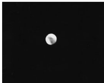
Figure 12.6 Defocused central diffraction spot from a small triangular-shaped silicon crystal. The out-of-focus diffraction pattern makes each diffraction spot into a low-magnification shadow image of the specimen, allowing simultaneous observation of the crystal orientation and position. As the specimen is tilted, corrections can be made to the translation controls to keep the same region of specimen in view.
