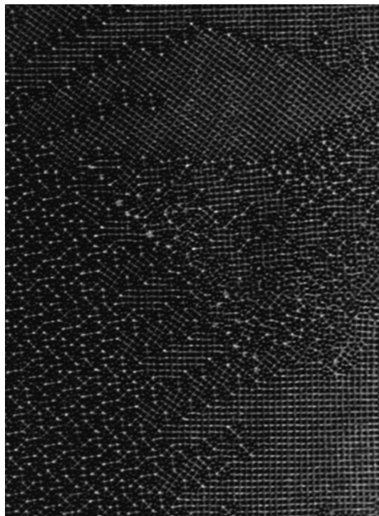
Figure 13.15 Solid state chemical reactions in action. HREM image along [001] of the in situ oxidation product of \text{Nb}_4\text{W}_{13}\text{O}_{47} , oxidized in an environmental cell under 20 mbar of oxygen. Domains of different structure appear as a result of the oxidation. Microdomains of \text{WO}_3 , tetragonal tungsten bronze, and disordered bronze structures can be identified. The instrument used was a modified JEOL 4000EX. (See Krumeich et al. (1999).)
