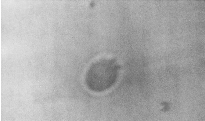
Figure 1.3 An image recorded under identical conditions to that shown in Fig. 1.2(a), with the laser source replaced with a tungsten lamp focused onto the object (critical illumination). The faint contrast seen is due to the preservation of some coherence in the illumination introduced by limiting the size of lens L2. This contrast disappears completely if a large lens is used. Variations in the size of this lens (or an aperture near it) are analogous to changes in the size of the second condenser aperture in an electron microscope.
