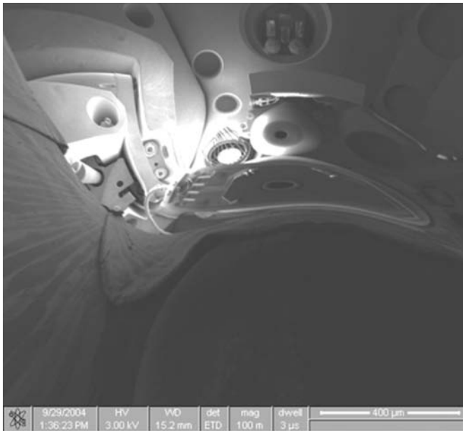
Figure 1.2 The ‘mirror effect’. Instead of landing on the specimen and forming an image of the specimen surface, primary electrons are repelled by the electric field arising from electrons implanted in the specimen, and turn back to strike the lens and other parts of the microscope. This generates signals that form an image of the inside of the chamber (distorted in this case)
