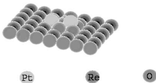
Fig. 6 Simplified model based on EXAFS data of \text{Re}_4\text{Pt}_2 clusters formed on the surface of \gamma\text{-Al}_2\text{O}_3 from \text{Re}_2\text{Pt}(\text{CO})_{12} [45]
