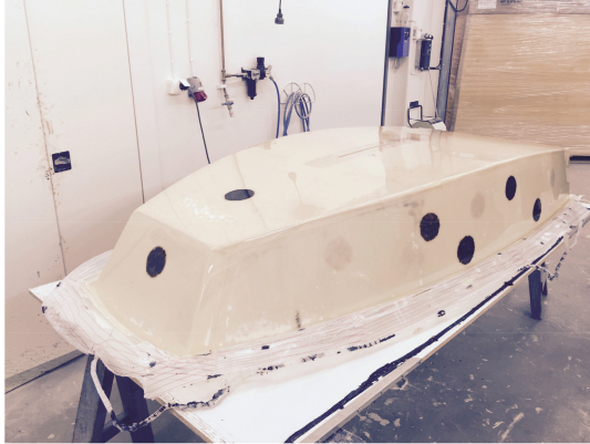
Fig. 1. An optimist built using a new bio-composite.
