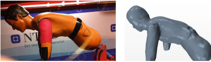
Fig. 3. Mannequin model in the wind tunnel (left) and 3D laser scanned model (right).
